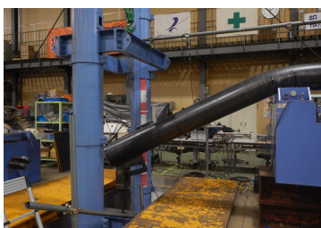
Full-Scale Static Load Test of the post
